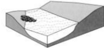
Structures that protrude from either streambank but do not extend entirely across a channel. They deflect flows away from the bank, and scour pools by constricting the channel and accelerating flow.
